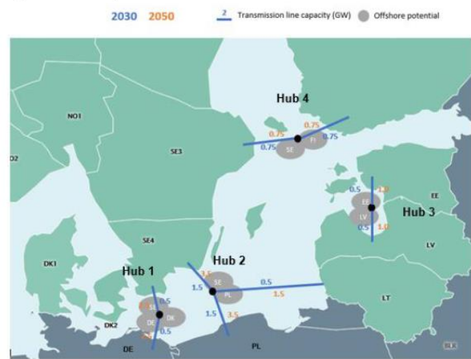
Figure 5-5 Configuration of the four advanced offshore hubs
